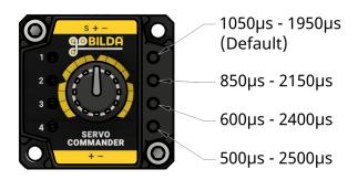
1050µs-1950µs is the default PWM range. This range allows most servos to rotate 90 degrees. Many servos are able to rotate further, given a wider range. If you purchased a goBILDA® Servo, reference the servo page for the maximum PWM range the servo is able to accept, and the corresponding rotation. This range is also used with goBILDA linear servos.
